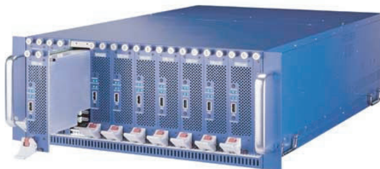
Figure 15: Inserting the FortiBlade-4010 module into the chassis
